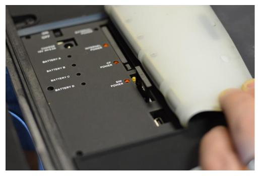
3. Install the SIM card and replace the SIM card carrier into the instrument.
